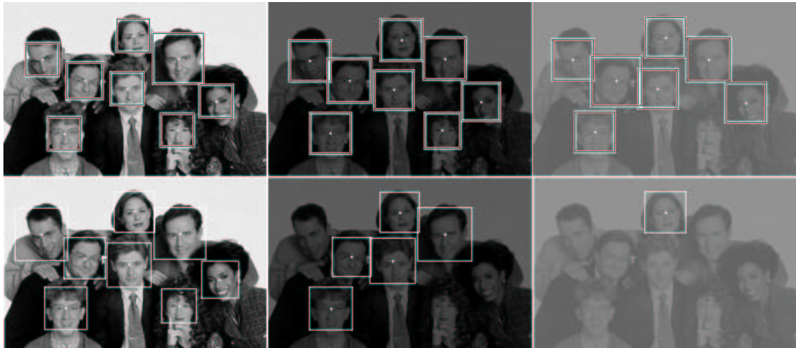
Figure 5. Contrast and brightness invariance for image transformations \Psi(\mathbf{I}) = a\mathbf{I} + b . Top row: Results using SNLTs. Bottom row: Results using a fixed threshold. Column one: Original image; Column two: a = 0.4 and b = 0 ; Column three: a = 0.2 and b = 100 .
