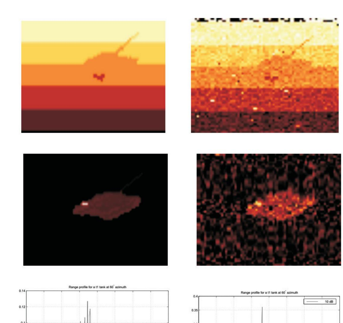
Shown in the left columns are LADAR, FLIR, and HRR data being studied in the Center for Imaging Science. Statistical sensor models have been characterized for LADAR, FLIR, and HRR and form the basis for optimum estimation. The LADAR likelihood is:
